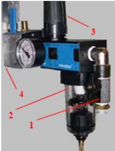
Input installation: [1] 12 mm tube / 1/2" fitting [2] Water separator [3] Regulator with manometer [4] Soft-start unit
